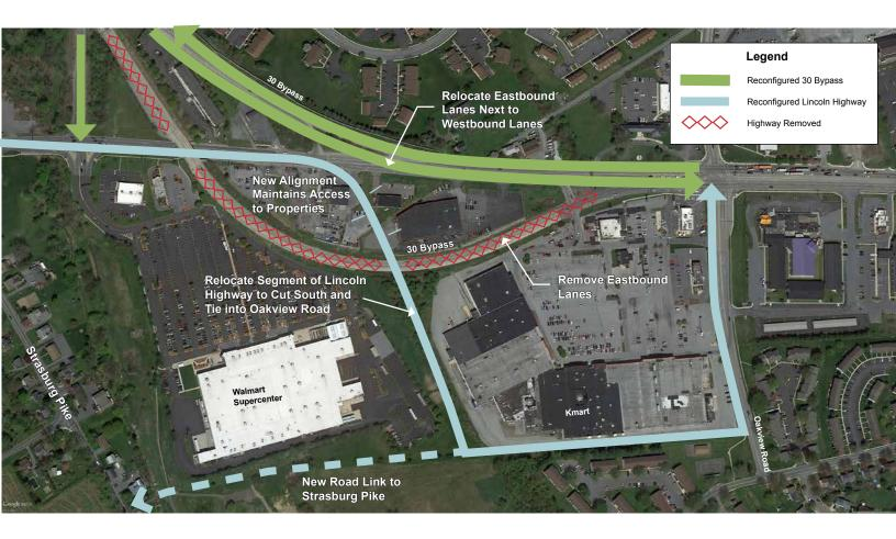
The full planned design of the Route 30 Bypass was never constructed, resulting in a partial Bypass ramp configuration, which presents safety and efficiency challenges for the corridor. A major reconfiguration of the roadway will be needed to fully address this issue. This planning process considered two potential alternatives to improve multi-modal access in this area.
