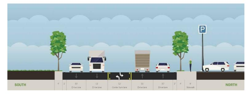
With a total ROW of 85 feet or less, a sidewalk is possible, but options are limited until the ROW reaches 78 feet. At 72 feet in width, the narrowest section, only the north side of the street would have a sidewalk in the ROW. On the south side, all sidewalk and/or multi-use trail facilities would need to be located on private property.
