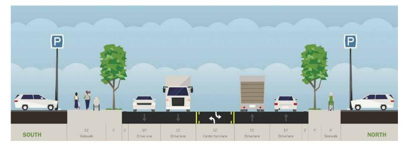
At 85 feet, the cross section can now contain all the elements of the roadway including the full width of the buffered multi-use trial on the south side of the road. As the ROW increases beyond 85 feet, space can be added to the landscape buffers.
